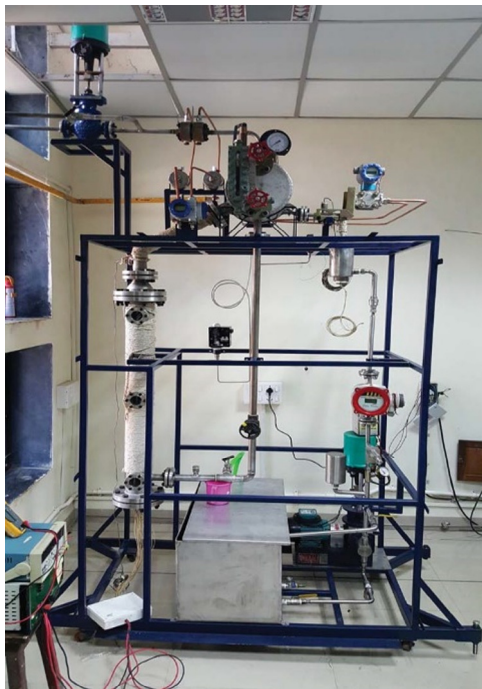
Fig. 2. Laboratory-scale boiler developed for research work.
