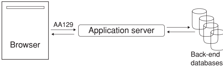
Figure 19.1 A dynamically generated web page. The browser sends a request for flight information on flight AA129 to the web application, which fetches the information from back-end databases then creates a dynamic web page that it returns to the browser.
