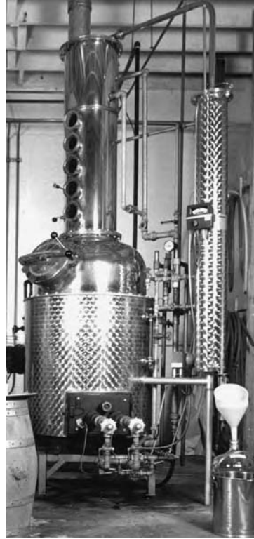
FIGURE 5.2 A continuous column still. In the version shown here, fermented mash (gray) enters the rectifier column and flows downward through a twisting pipe surrounded by superheated steam. This hot mash is then pumped to the top of the analyzer column. Here it steeps down through perforated plates, meeting superheated steam entering from the bottom of the rectifier. There they rise again through perforated plates condensing as they are cooled by the mash descending in the twisting pipe. Then the condensed spirits are drawn off at their desired degree of alcohol content. Photo courtesy of Clear Creek Distillery, Portland, Oregon.
