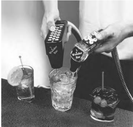
FIGURE 4.5 Handguns for a soda system. Photo courtesy of Wunder-Bar Automatic, Controls, Inc., Vacaville, California.
