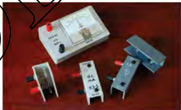
Figure 2.35 Shunts and multipliers for use with a galvanometer
