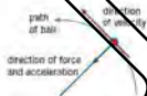
Figure 7.3 A ball swung in a circle on the end of a string
