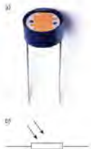
Figure 19.2 An LDR and its schematic.
