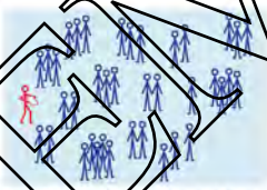
Figure 19.11 The wider the wire, the easier it is for the charges to pass through.
