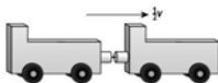
The two trolleys stick together and move off with a combined speed of \frac{1}{2}v .
