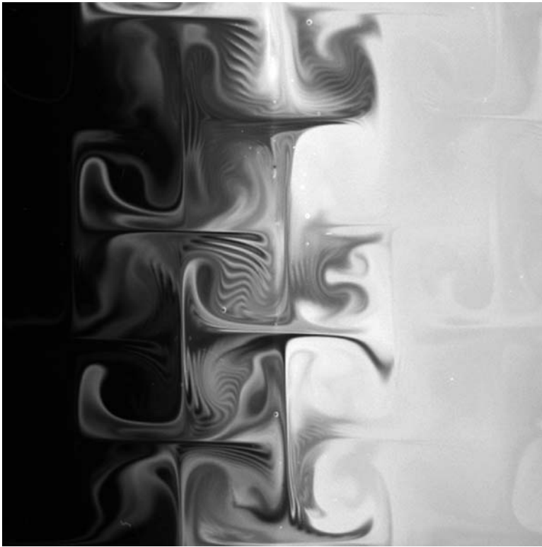
Fig. 3.5 Fluid labelled with fluorescein was initially confined to the right half of a cell. Forcing occurs by a time-periodic electric current in the presence of a spatially periodic magnet array. The repetitive stretching and folding that is characteristic of chaotic advection is evident. [Reprinted from Rothstein et al. (1999) with permission from Macmillan Publishers Ltd.]
