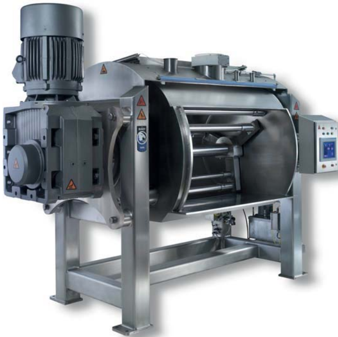
Plate 5.3 Industrial bread dough mixer. (Courtesy of Shaffer Manufacturing.)
