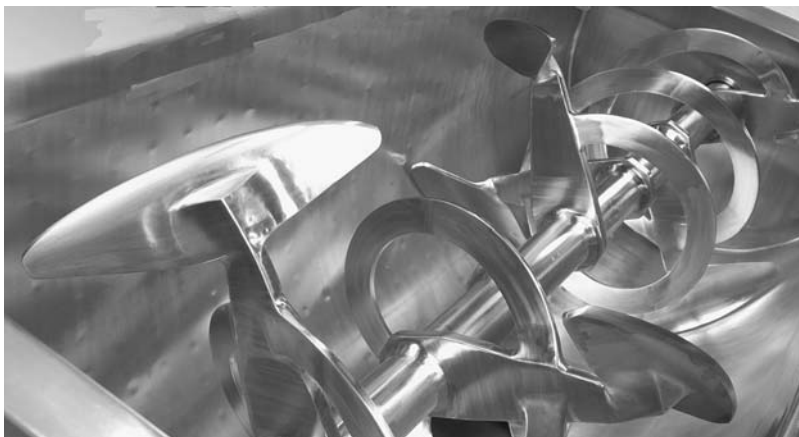
Fig. 5.7 Combination ribbon–paddle agitator. (Courtesy of American Process Systems, Eirich Machines, Inc.)
