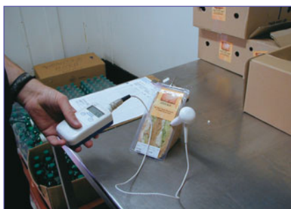
Figure 16.20 Temperature control (a): checking chilled temperature
