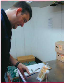
Figure 7.8 A delivery temperature recorder, which gives a printout of data
