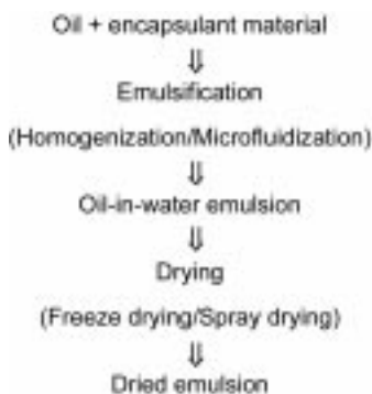
Fig. 15.1 Generalized process for production of dried oil-in-water emulsions.
