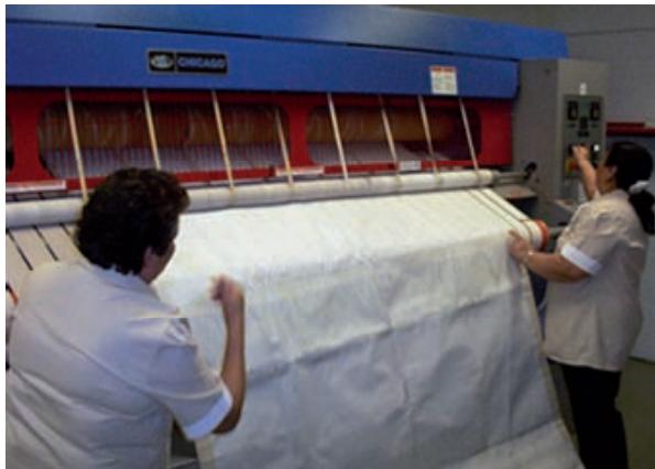
Figure 5.7: Linen/laundry room employees operating a 'flatwork ironer'
