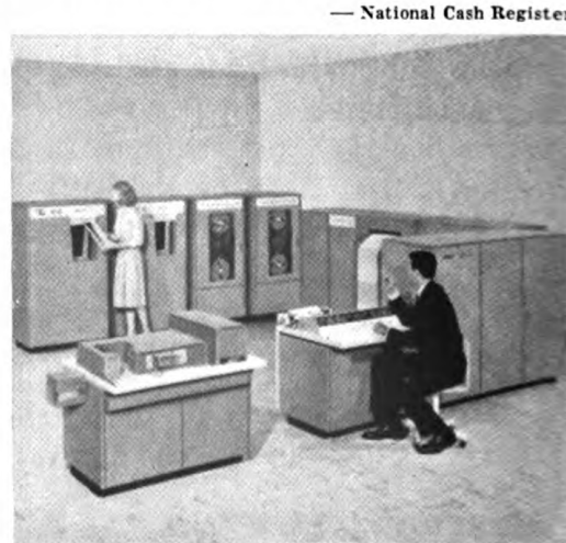
Fig. 127. Magnetic cards are placed in the Card Random Access Memory Unit of a data-processing system.
