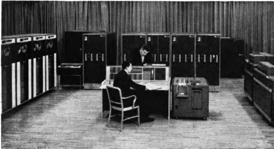
Fig. 67. A data processing system for controlling and feeding instructions to machine tools.
