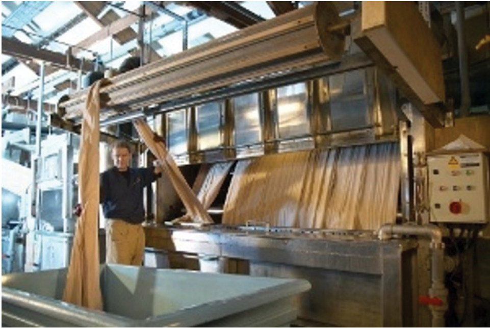
Figure 4.20 Winch dyeing machine for multiple lengths of fabric (Source: Photograph courtesy of DP Dyers, Holmfirth, UK).
