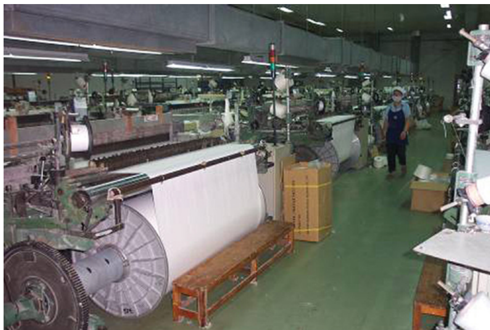
Figure 2.21 Rear view of a loom showing the beam and warped threads.
