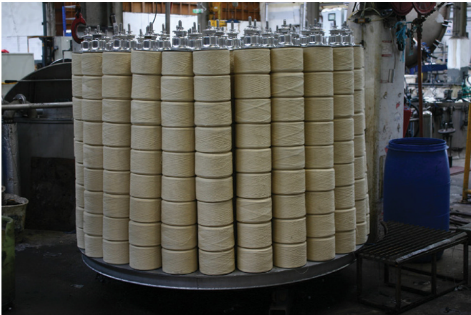
Figure 4.14 Packages of wool yarn on the spindles of a package dyeing machine of 900 kg capacity (Source: Photograph courtesy of Bulmer and Lumb Group, UK).
