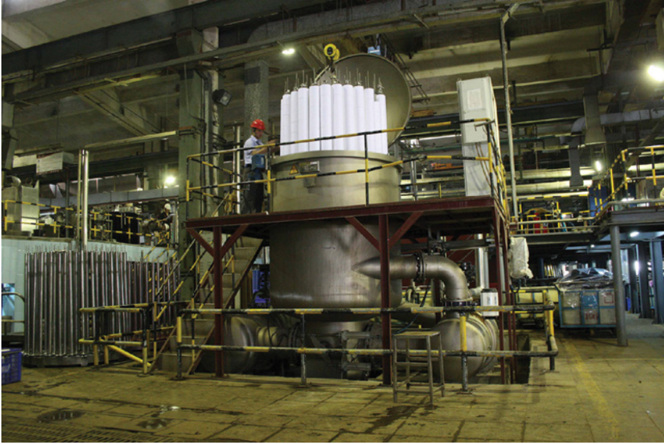
Figure 4.15 Loading a package dyeing machine (Source: Photographs kindly supplied by Thies GmbH & Co. KG, Germany).
