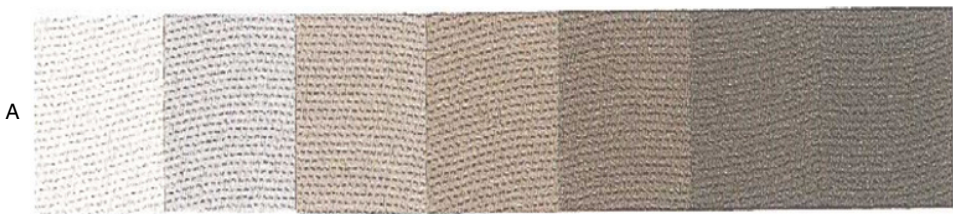
Figure 4.5 On-tone build-up of a trichromatic mixture of direct dyes belonging to the same class.
