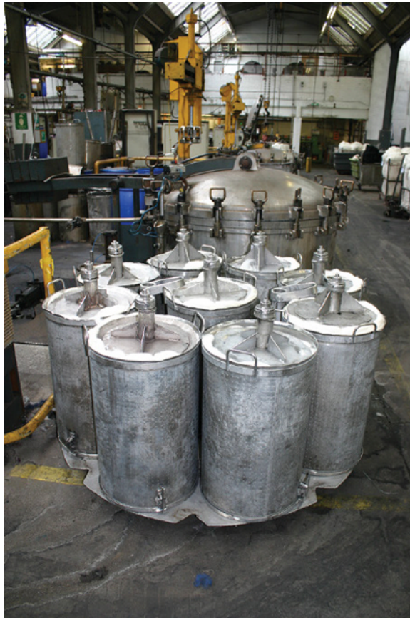
Figure 4.11 Nine cages, each containing five bump tops, ready to be hoist into the dyeing machine (Source: Photograph courtesy of Bulmer and Lumb Group, UK).
