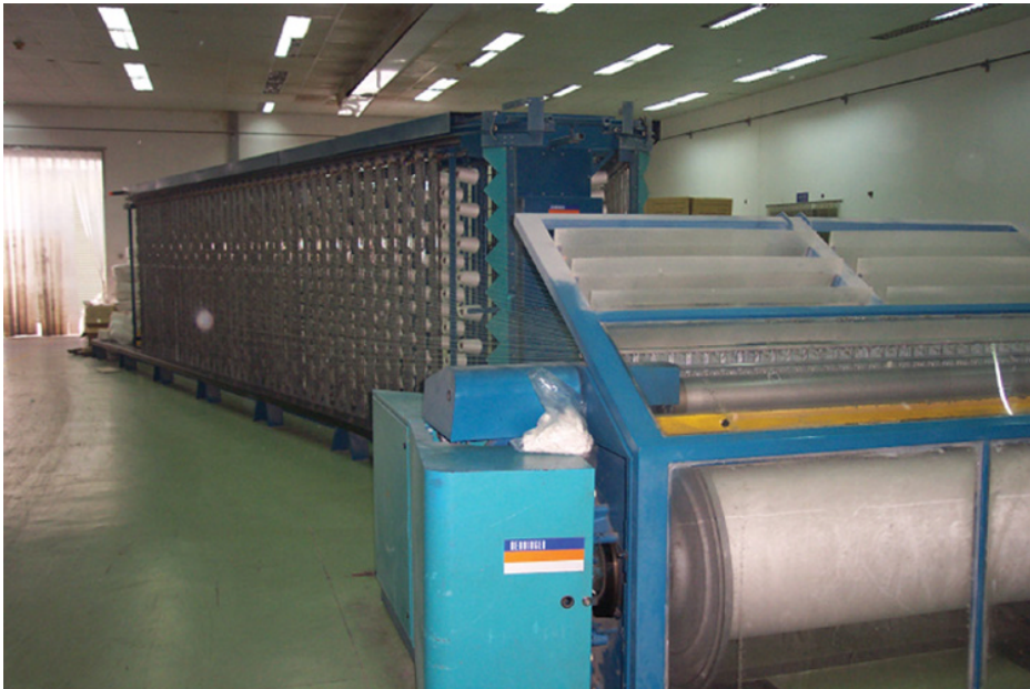
Figure 2.20 Winding from bobbins on to a beam.
