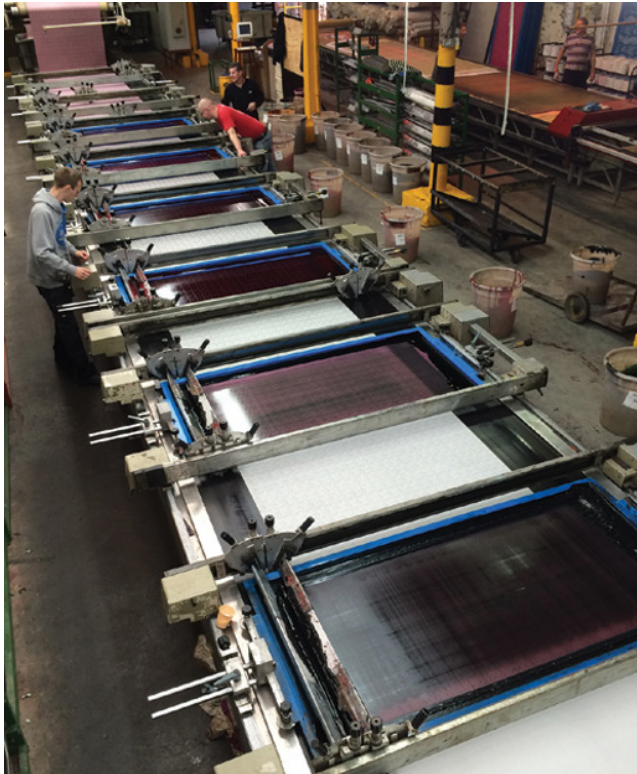
Figure 5.8 Commercial flat screen printing (Source: Photograph courtesy of Standfast and Barracks Ltd., Lancaster, UK).
