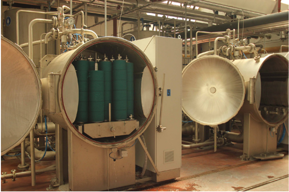
Figure 4.16 Horizontal loading package dyeing machine (Source: Photographs kindly supplied by Thies GmbH & Co. KG, Germany).
