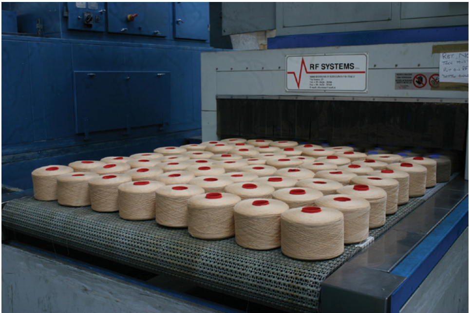
Figure 4.17 A radio-frequency drying machine (Source: Photograph courtesy of Bulmer and Lumb Group, UK).
