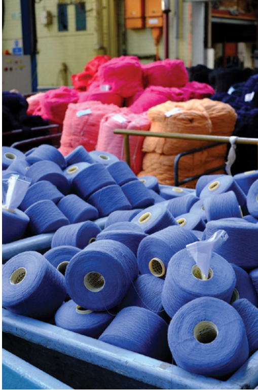
Figure 4.13 Cheese packages on rigid plastic formers, after dyeing. In the background are dyed wool tops (Source: Photograph courtesy of Bulmer and Lumb Group, UK).
