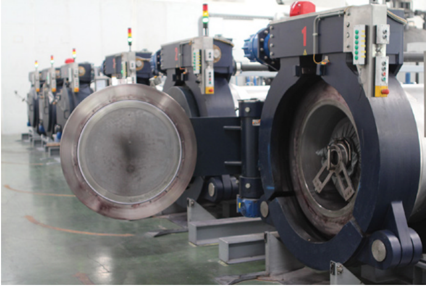
Figure 4.30 DyeCoo scCO 2 beam dyeing machines installed at Yeh Group factory in Thailand (Source: Reproduced by kind permission of the Yeh Group).
