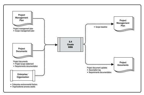
Figure 5-11. Create WBS: Data Flow Diagram
