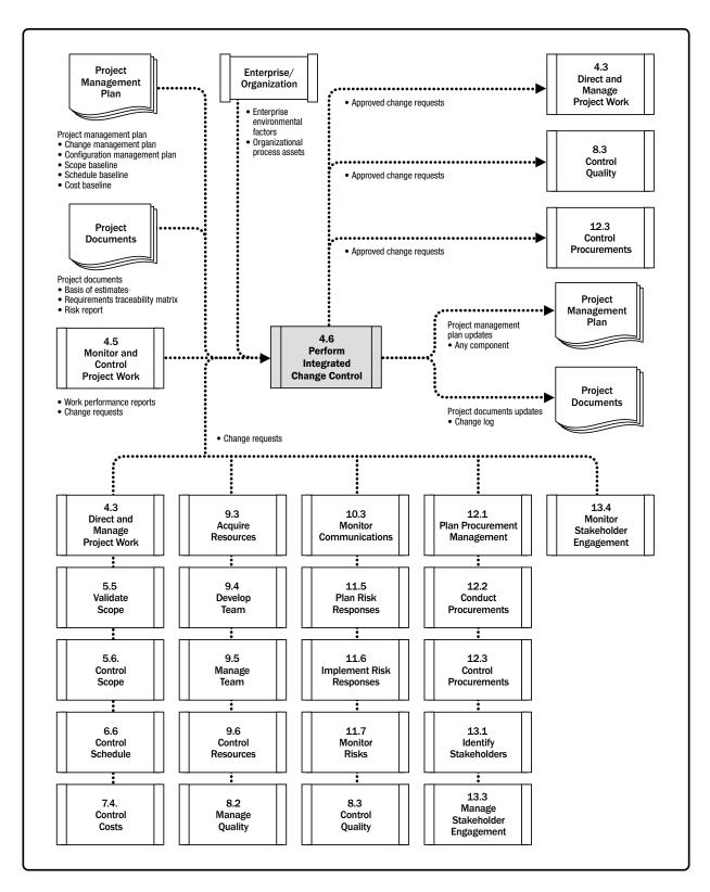
Figure 4-13. Perform Integrated Change Control: Data Flow Diagram
