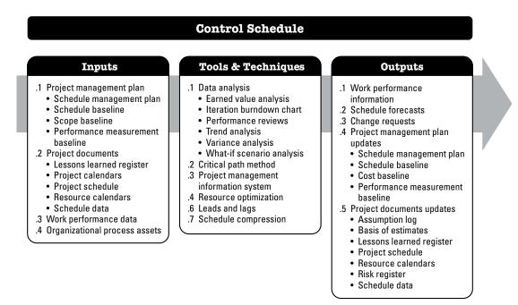
Figure 6-22. Control Schedule: Inputs, Tools & Techniques, and Outputs
