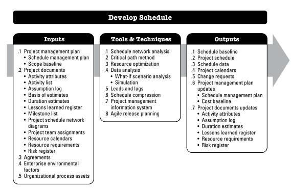
Figure 6-14. Develop Schedule: Inputs, Tools & Techniques, and Outputs
