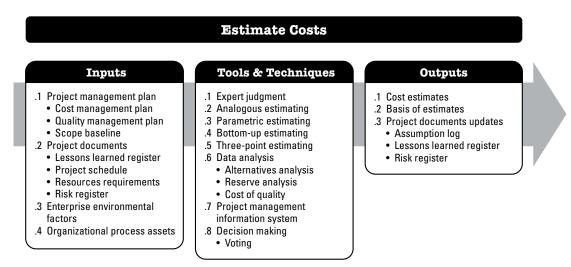
Figure 7-4. Estimate Costs: Inputs, Tools & Techniques, and Outputs
