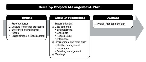
Figure 4-4. Develop Project Management Plan: Inputs, Tools & Techniques, and Outputs
