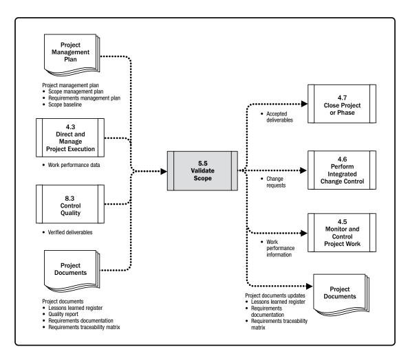
Figure 5-16. Validate Scope: Data Flow Diagram
