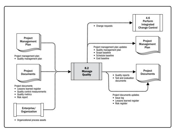
Figure 8-8. Manage Quality: Data Flow Diagram
