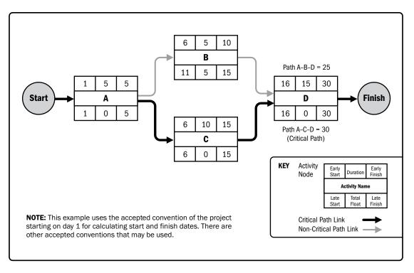
Figure 6-16. Example of Critical Path Method
