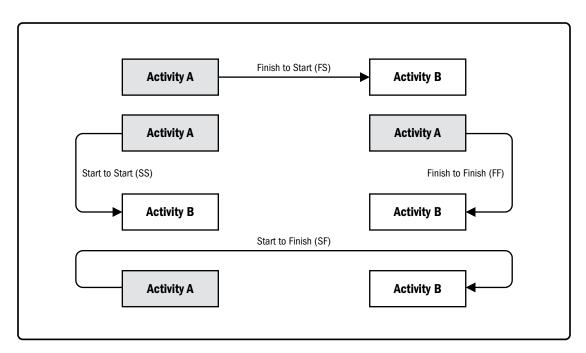
Figure 6-9. Precedence Diagramming Method (PDM) Relationship Types
