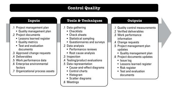
Figure 8-10. Control Quality: Inputs, Tools & Techniques, and Outputs
