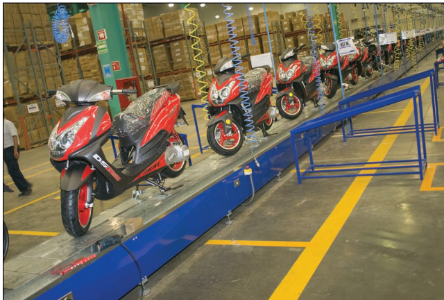
A repetitive process: Motorcycles on an assembly line with parts added in a sequential order.
