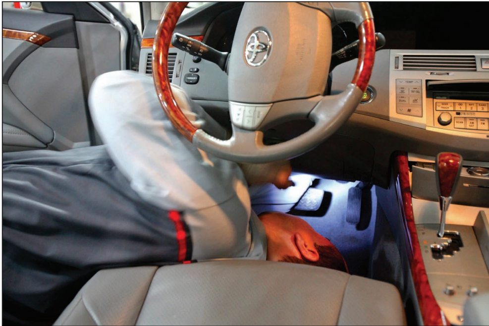
A Toyota technician prepares to remove the accelerator assembly in a recalled Avalon.
