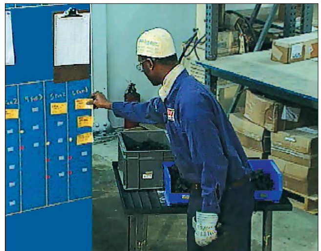
Special carts were designed that, when filled, act as a visual signal that they are ready to be moved to the next work cell. An empty cart indicates that it is time to produce, in order to refill the cart.
