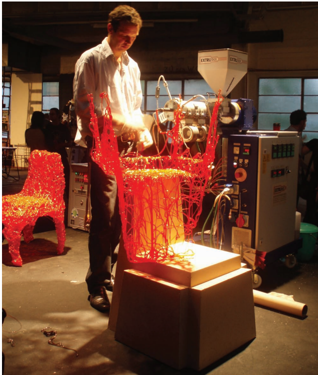
A microfactory consisting of an Extrudex machine, which produces fluid tubes of plastic (extrusions) that are turned into designer chairs.
