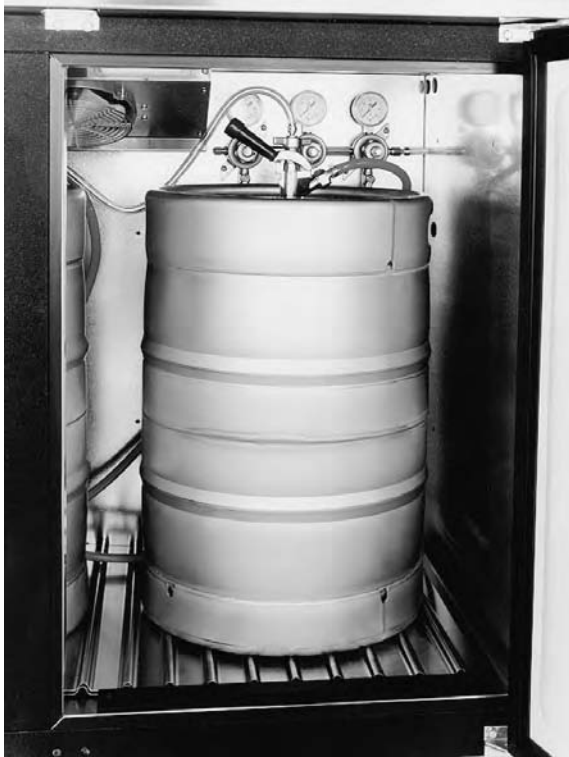
FIGURE 8.11 A self-contained system. Dark lines carry beer from keg to tap. Light lines carry carbon dioxide to keg. Cylinder (not shown) is outside refrigerator at room temperature. Courtesy of Glastender, Inc., Saginaw, Michigan.
