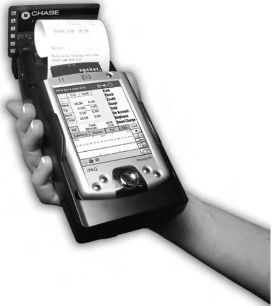
FIGURE 14.13 A hand-held POS unit allows transactions to be made and receipts to be printed without the server leaving the table. Courtesy of Action Systems, Inc., Silver Spring, Maryland.
