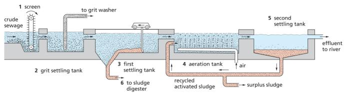
Figure 21.35 Sewage treatment – activated sludge process
