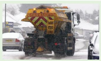
Figure 3.17 Salt gritter at work to prevent ice formation on a road
