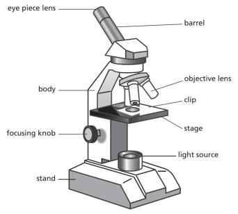
Figure 2.17 A light microscope
